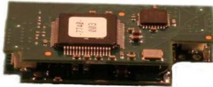
(TS//SI//REL) FLUXBABBITT Hardware Implant for PowerEdge 2950
