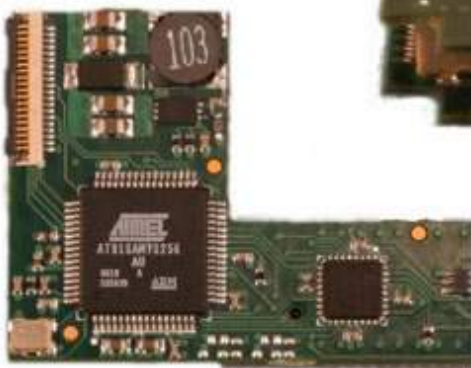
(TS//SI//REL) FLUXBABBITT Hardware Implant for PowerEdge 1950
